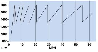
Based on 1800 RPM engine operating at 1550 RPM/62 MPH.
